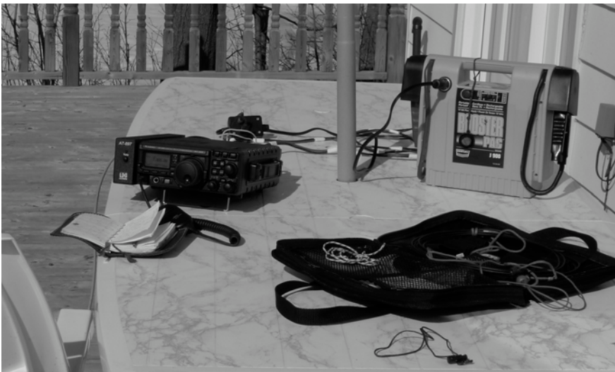
Portable HF station Yaesu FT897 and booster battery power supply.
