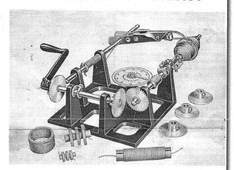
This new, hand-operated, coilwinding machine will produce self-supporting, universal and honeycomb coils, also solenoid, single-layer, etc. Samples of these are illustrated.
