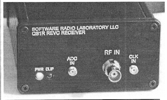
Bottom right picture shows the 2008 QuickSilver 1 SDR Receiver. All the signal processing is done by mathematics. The unit attaches to your computer with a USB cable and is controlled using a software interface. Performance is noticeably better than traditional receivers. It sells for around $1000.
