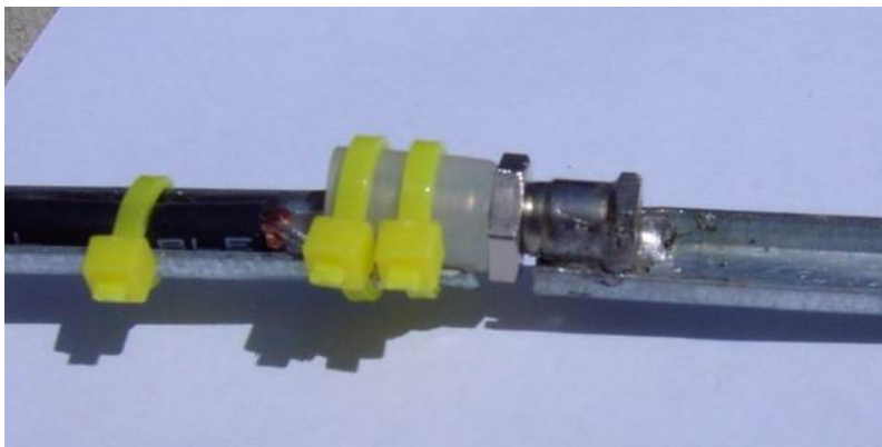
Figure 7 – The Driven Element is attached to the boom with a #10-24 machine screw with a wingnut. Note that the coax cable is tied wrapped to the driven element right up to the boom, where the RF voltage is zero.
