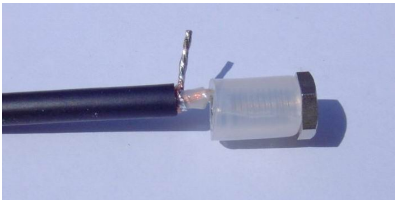
Figure 3 – Slide the polyethylene tubing insulation over the jack.
