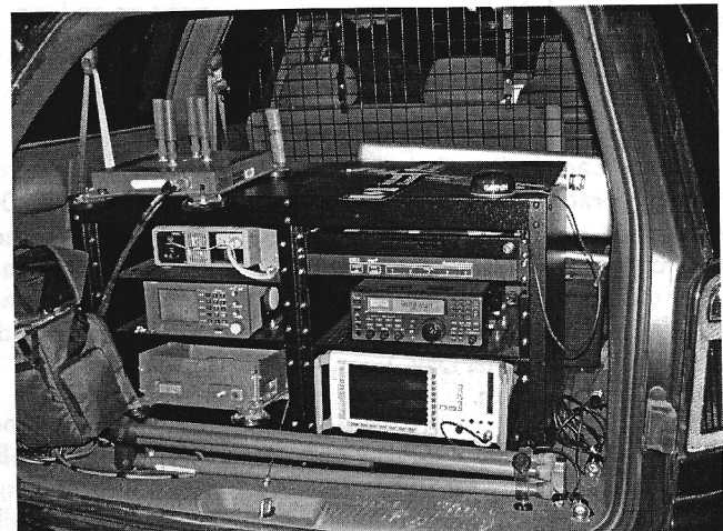
Above, a look inside the back of the MIRS van which is packed with specialized equipment including a spectrum monitor, power supply, multimode receiver, radio direction finding receiver, and land mobile communication transceiver. Nice stuff!
